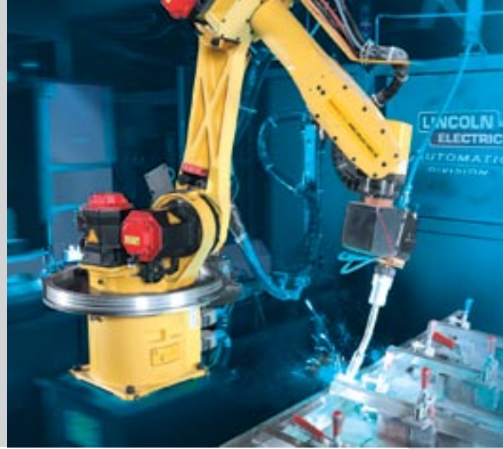
Pre-Engineered Automation System: Fanuc ArcMate Robot with Lincoln Electric Welding Package, featuring the Balluff zone limit system.
